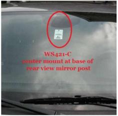
**Center Mounting** the tag at the bottom of the rear-view mirror post works nicely when the Readers are mounted directly overhead in the center of the lane. This is also the recommended position when a combination of Windshield Stickers and Hangtags are being used.
